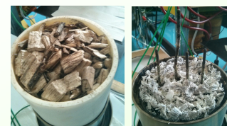
Fuel and residues (ashes) from a test run with beech wood chips
