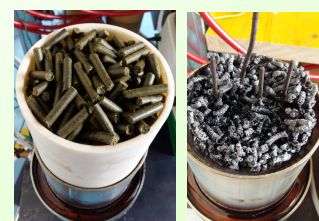
Fuel and residues (ashes) from a test run with straw pellets
