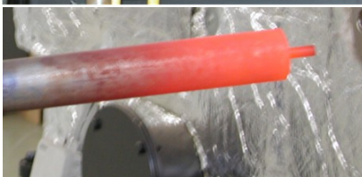
High temperature impactor immediately after sampling
