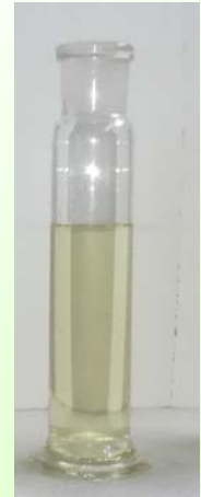
Isopropanol solution with tars sampled downstream the catalyst
