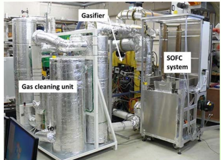
Biomass gasifier coupled with a solid oxide fuel cell (SOFC) system 6 kW el testing plant at BIOS
