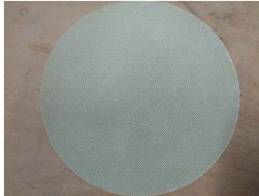
Wire-Mesh catalyst for tar reforming
