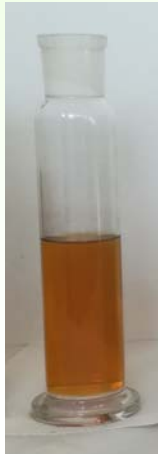
Isopropanol solution with tars sampled upstream the catalyst
