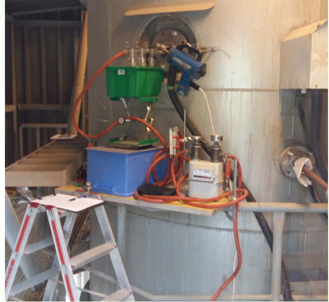
Gas sampling during a test runs at a biomass combustion plant
