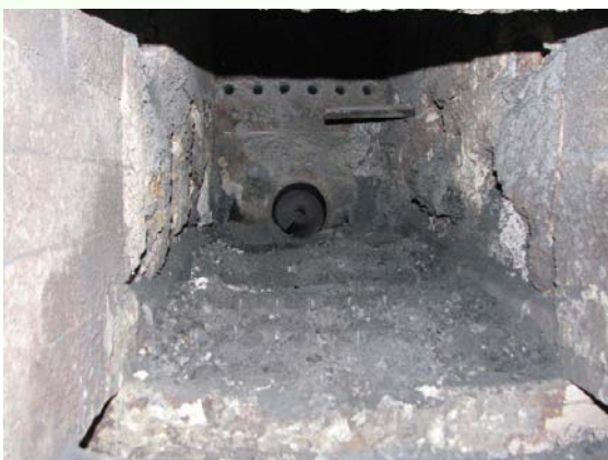
Molten ash agglomerations formed during the combustion of herbaceous fuels
