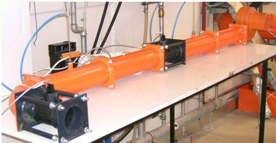
Testing stand for the evaluation of the performance of different devices from the determination of flue gas and air velocities
