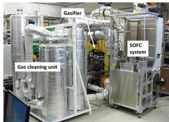
**Figure 5:** Picture of the testing plant located at BIOS
