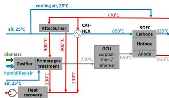
**Figure 2:** Flow diagram of the HiEff-BioPower CHP technology
