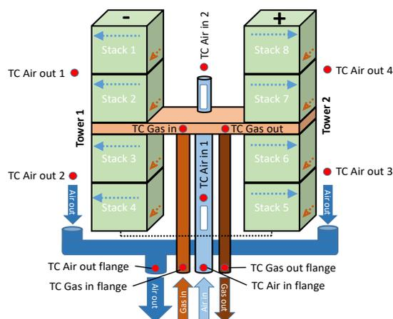
**Figure 9:** Schematic drawing of the stack module
