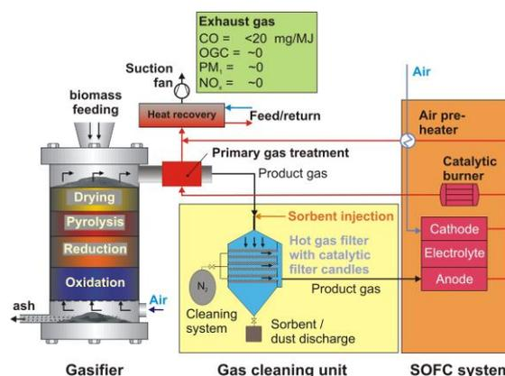
**Figure 1:** Scheme of the HiEff-BioPower technology
