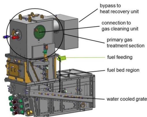
**Figure 5:** 3D-drawing of the new updraft gasifier
