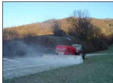
Figure 4: Ash spreading with a screw spreader [11]
